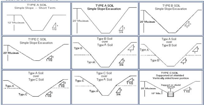
ANGLE OF REPOSE: Stable Rock-90; Type A Long-53; Type B-45; Type C-34
